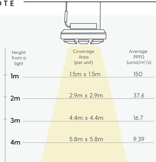
To build PPFD levels, multiple lights should be utilised and arranged in a layered set up. Contact the Telos team for more information.
